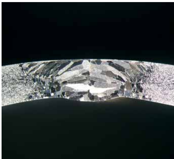
Text to Fig. 3: Macro image, overview of relatively wide TIG weld seam 1.4521
