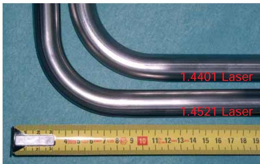
Text to Fig. 5: Pipe with the dimension 22x1,2, bent with r = 2.5 \times d , result: 1.4521 no difference to 1.4401
