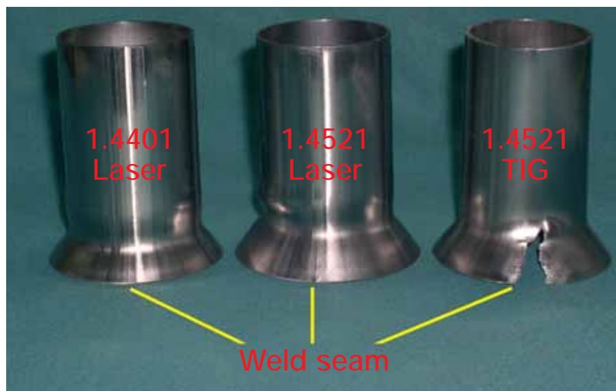
Text to Fig. 6: Comparative flaring tests, laser welding for 1.4401 and 1.4521 ideal, the TIG weld of 1.4521 with crack through grain coarsening
